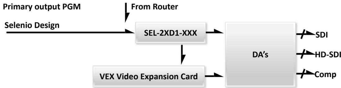
Using Selenio for utility and transmission chain processing streamlines a previously complex architecture and workflow. Card count is reduced by a factor of up to five or six, wiring is simplified and router I/O counts are reduced. The result is significantly reduced rack space, improved flexibility and faster setup.
