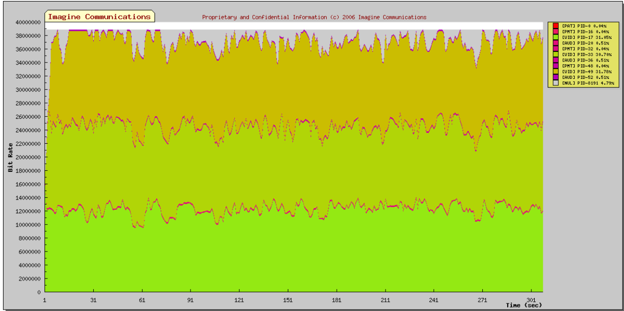
Figure 3: Three (3) HD-VOD VBR Streams in 256 QAM Channel
